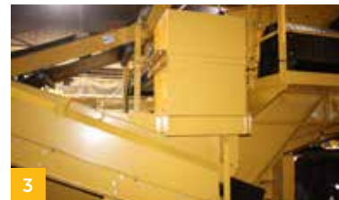
3 Ability to return top and bottom deck oversized material back to the crusher. This feature increases production by splitting the load on two decks rather than one.
