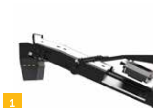
1 36" main conveyor as standard, giving large stockpile capacity. Conveyor lowers and raises hydraulically.
