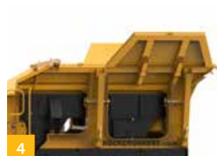
4 Folding HARDOX® hopper mounted over vibrating pan feeder built with steeper angles to reduce material sticking. Feeder rate regulated manually or automatically by load sensing jaw.
