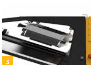
3 Optional overband magnet enables magnetic material separation from the source material.
