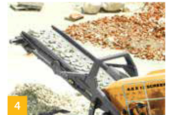
4 Discharging oversize material at 11'-4" (3.45 m), the 48" (1200 mm) wide 3-ply belt allows for efficient stockpiling.
