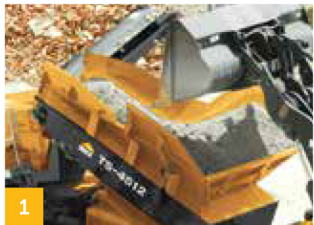
1 7.8 yd 3 (6 m 3 ) hopper equipped with a 48" (1200 mm) heavy duty 4-ply belt designed for heavy duty applications.
