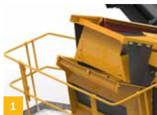
1 42" (1200mm) feed conveyor enables high capacity screening.
