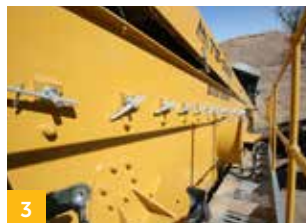
User friendly wedge system ensures faster screen changes.
