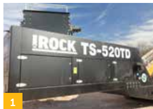
15' (4267mm) grid opening allows the use of larger loading shovels.
