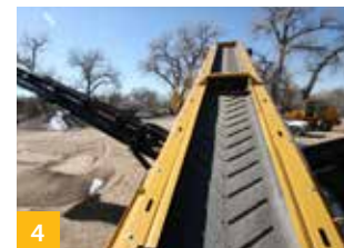
42" (1200 mm) feed conveyor enables high capacity screening.
