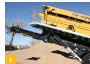
Hydraulic Screenbox linkage system, allows greater accessibility for screen change and enables optimum screen coverage at varying screenbox angles.
